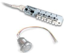
The X-Touch button interface is a 4-channel push-button interface with LED control and can be used in combination with industry-standard push buttons. It allows the connection of up to four buttons onto a single interface. This results in the connection possibility of up to 9 push buttons even on the smallest Xperience controller. Programmable LED output options are on, off, slow and fast blink.
