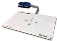
The XT-EF series sensors can detect AirButtons, AirGestures and AirWheels. AirButton detects whenever a person's hand enters and leaves the sensor's detection field and can also register and respond to physical Touch input. AirGesture registers left, right, up, and -down swipes within the detection field. AirWheel detection processes circle tracing by the user's fingers above the sensor.
