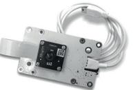
The X-Eye Gender sensor detects the gender and age range of a person, enabling content triggering and data collection. It does not require network connectivity and doesn't store video data, making it 100% GDPR-compliant.
